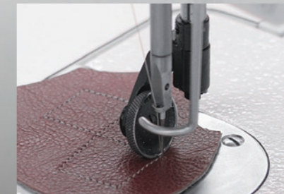
PFAFF 2083-8/44: Special version with roller foot for basic shoe applications
