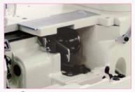
Swing in and out looper thread take-up for easier threading.
