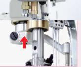
Spreader holder has alignment mark. Reinstathe spreader is easy.
