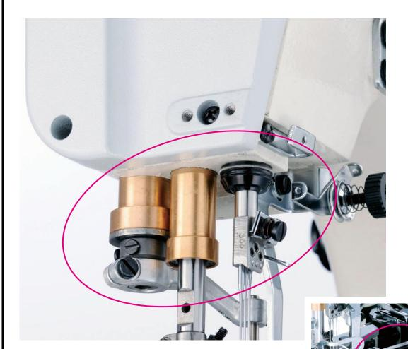
\*Looper shaft can be equipped with only for W600P series.
